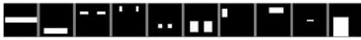
Figure 4. Some of LDA guided OOMP selected box functions to approximate the first binary LDA base vector.
